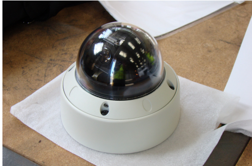
Security surveillance camera engineered for attachment to underwing inspection cover.
